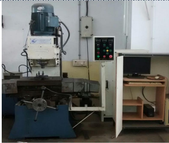
Fig. 1: Friction Stir Processing Setup used in this study
